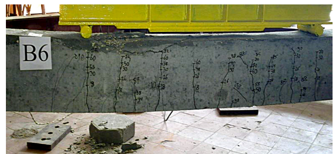
Fig. 7 Typical flexure failure for the beam specimens.
