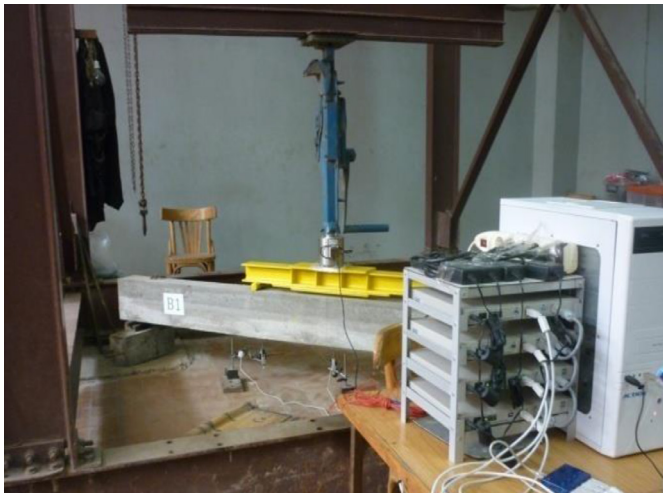
Fig. 4 Splice beam prior to the testing.
